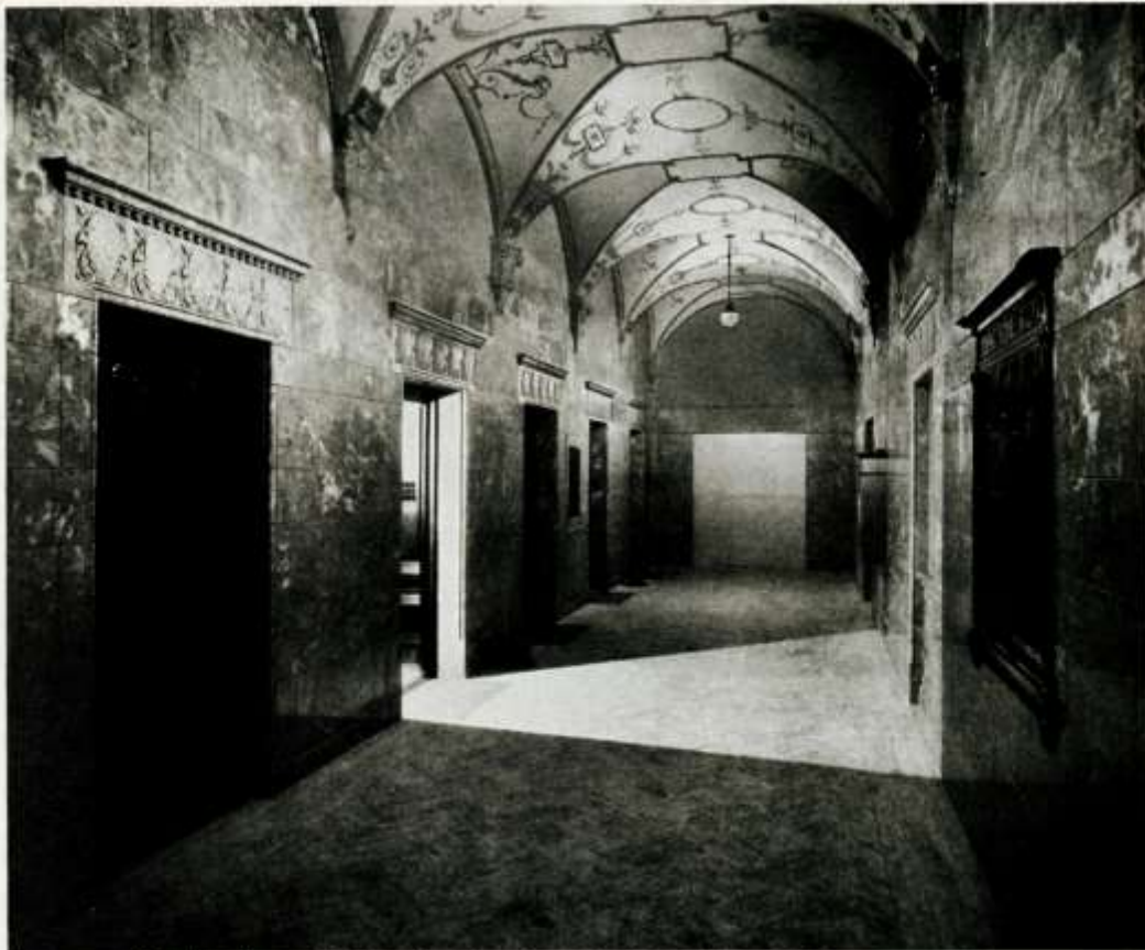
Pershing Square Building, Los Angeles, Cal. The walls are St. Genevieve marble, the floor Travertine. Curlet and Beelman, architects.
