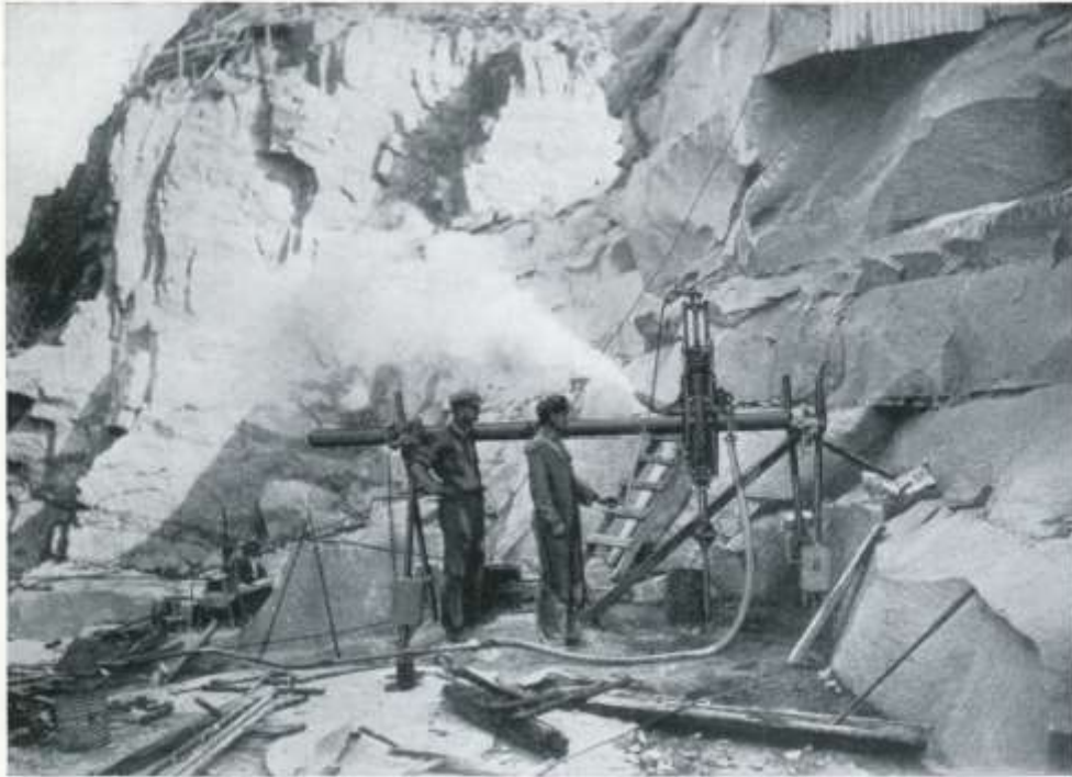
A corner in the Smith Granite Co. Quarry showing the Sullivan "UH" Drill and Quarry Bar
