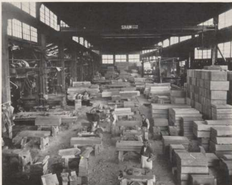
Interior Main Runway, showing cutting department of the cut stone plant of H. J. Horner & Sons, Newark, N. J.
