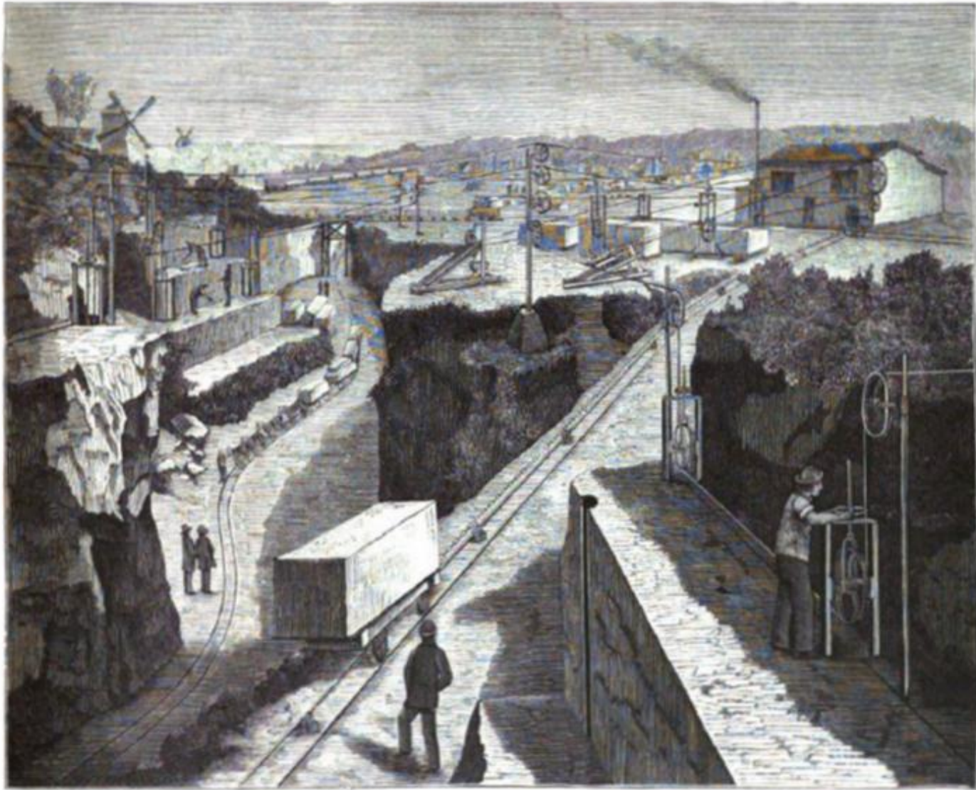
APPLICATION OF GAY'S STONE SAW IN A MARBLE QUARRY.
