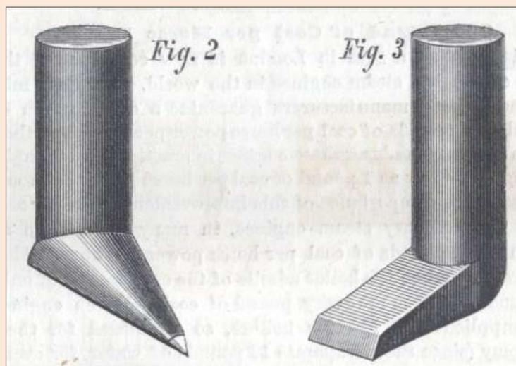
“These cutters strike no violent blows, to fracture the stone or make breaks or holes in its surface. Their motion is so slow as not to heat the tools, but so forcible as to enter the hardest limestone, or marble. When cutting granite, by the use of tools armed with carbon points, the speed is increased one hundred times, cutting down a ‘rough’ of three inches, and throwing it off in the form of impalpable powder.
