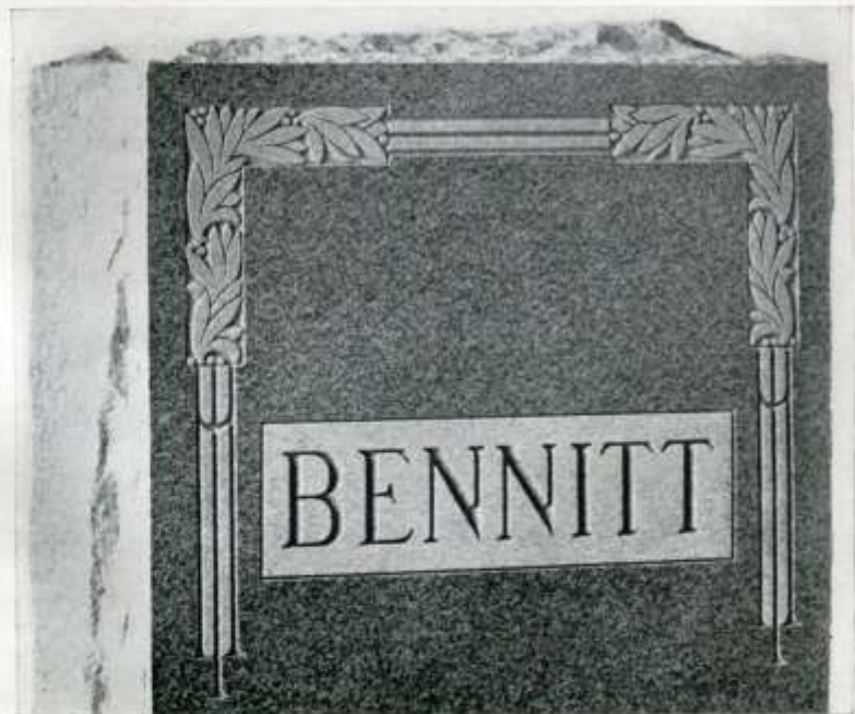
FIG. 7. FLAT CARVING AND SUNK LETTERING, SHOWING BEAUTIFUL EFFECTS WITH SAND BLAST Work of Slaughter-Thompson Co., South Bend, Ind.
