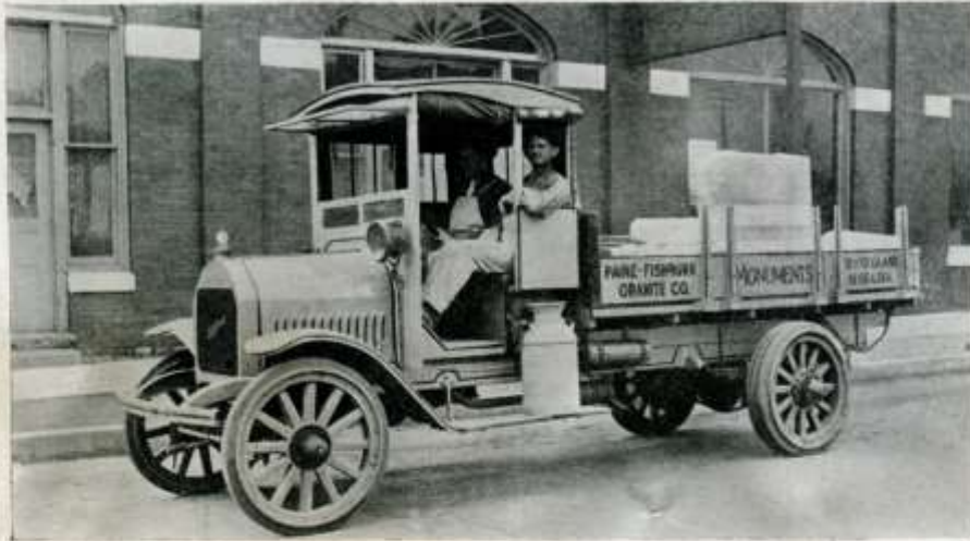
TWO-TON LITTLE GIANT TRUCK USED BY PAINE-FISHBURN GRANITE CO., GRAND ISLAND, NEBRASKA, EQUIPPED WITH SOLID TIRES.
