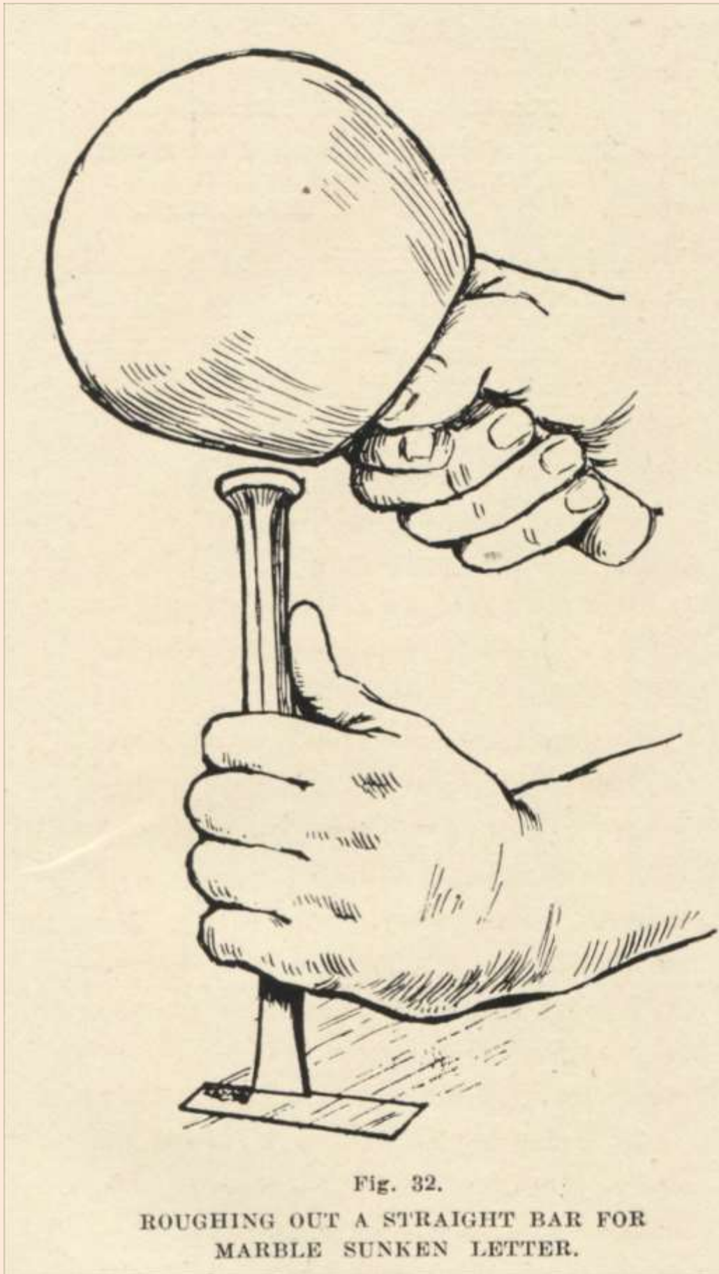
Fig. 32. Roughing out a straight bar for marble sunken letter
