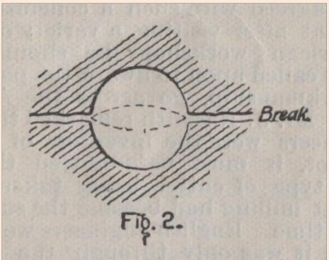
"It was found that with the old Portland canister two breaks might be made at right angles by a single blast, when using a canister shaped like a square prism. In some of the larger blasts, where blocks weighing in the neighborhood of 2,000 tons were sheared on the bed, two holes as deep as 20 ft. were drilled close together. The core between the holes was then clipped out and large canisters measuring 2 ft. across from edge to edge were used.
