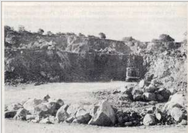
FIG. 13. J. M. Nelson quarry. Rock is olivine basalt in flat-lying flows associated with tuffs and breccia. The basalt is now being quarried for crushed rock. Formerly used in making paving blocks.
