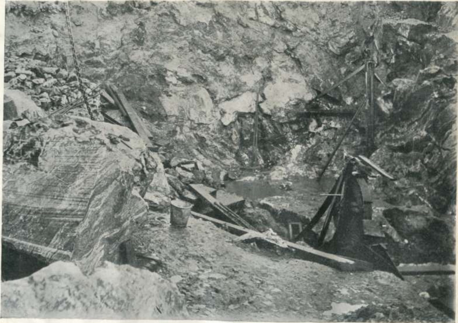
WIRE SAW AT WORK IN THE GALWAY MARBLE QUARRY.
